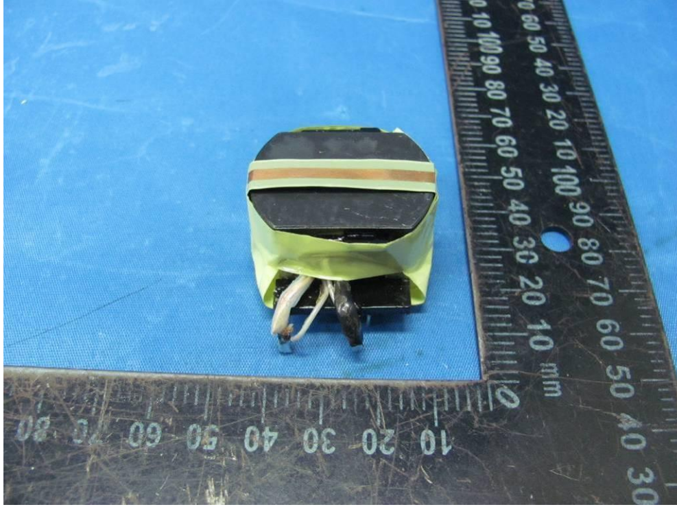
GT*41133 series Primary winding view of mains transformer
