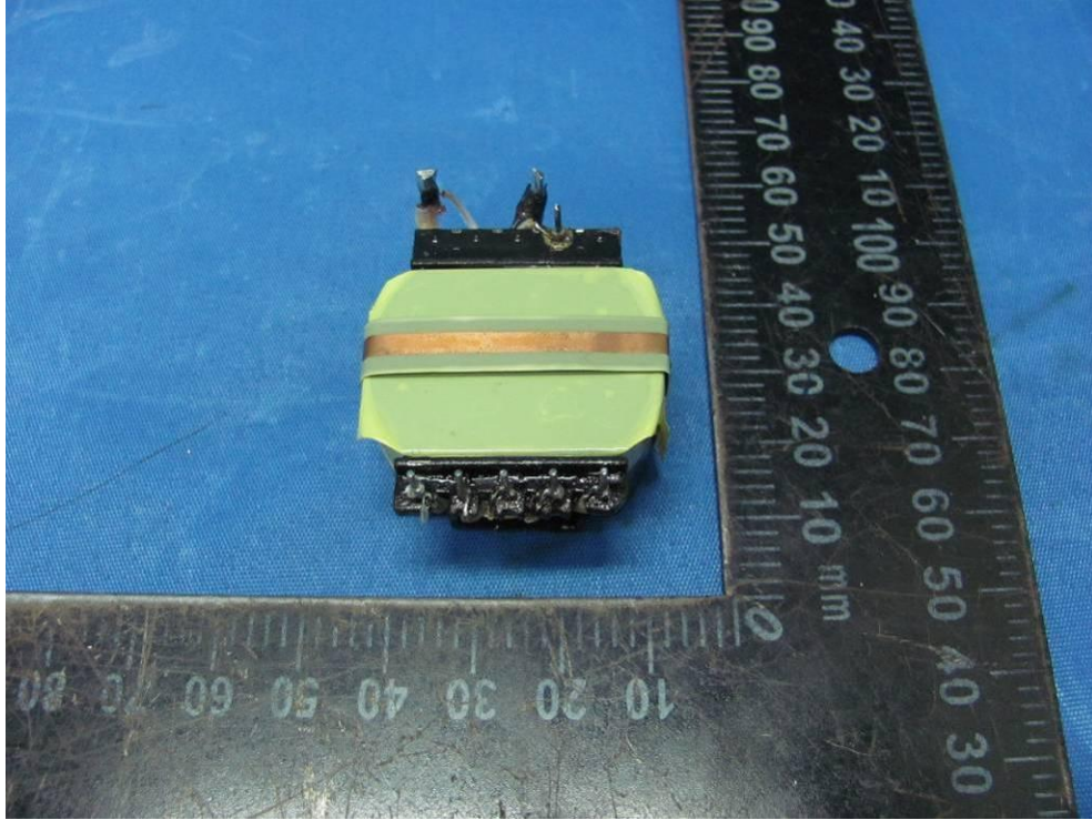
GT*41133 series Bottom view of mains transformer (The ferrite core is wrapped around 2 layers of insulating tape.)
