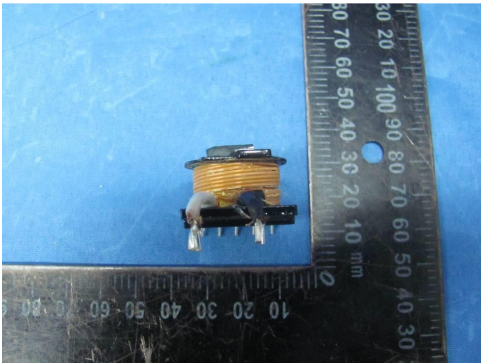
GT*41133 series Secondary winding view of mains transformer (TIW)
