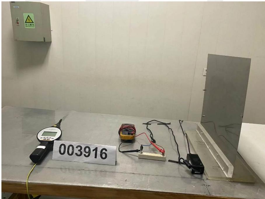
16.5.Photo of Continuous RF Electromagnetic Field Disturbances
