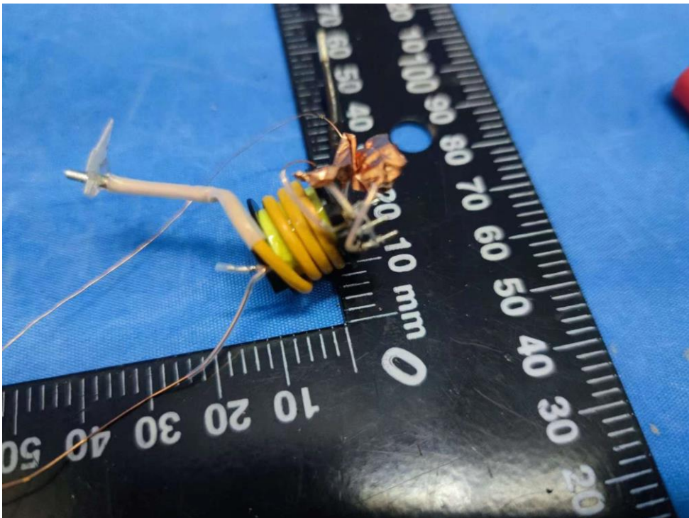
Transformer view of TF103
