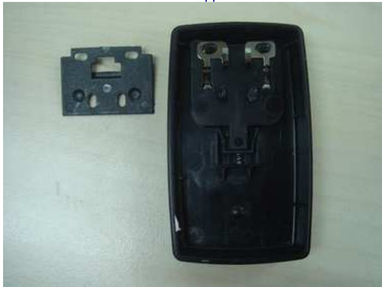
Internal view of appliance inlet
