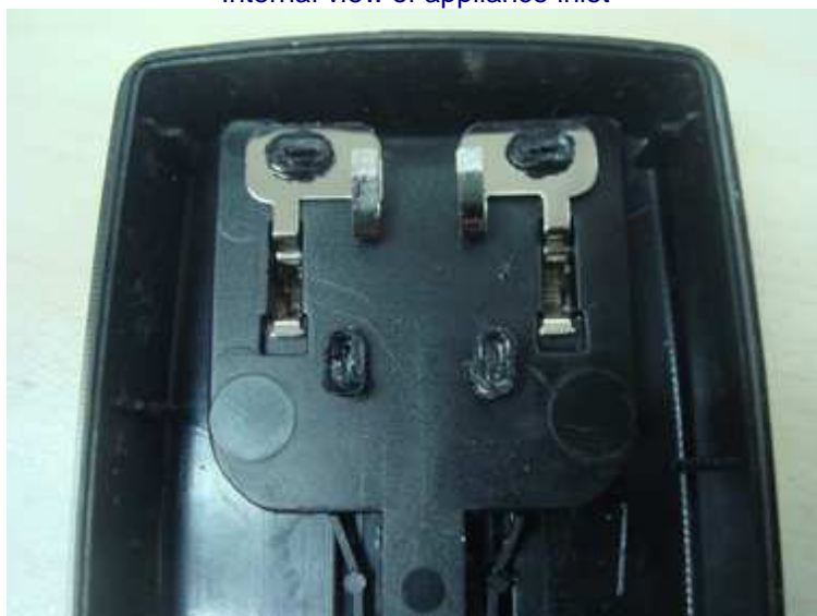
Internal view of appliance inlet
