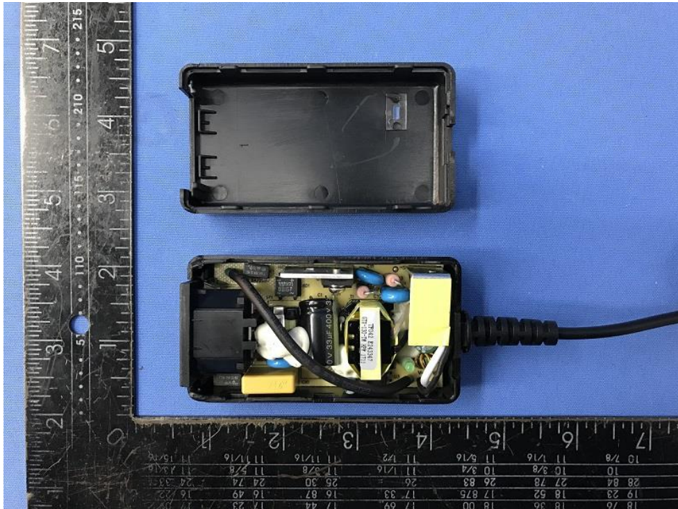
PCB view for GTM96180 series (Class I) with R22, R23 and without R24
