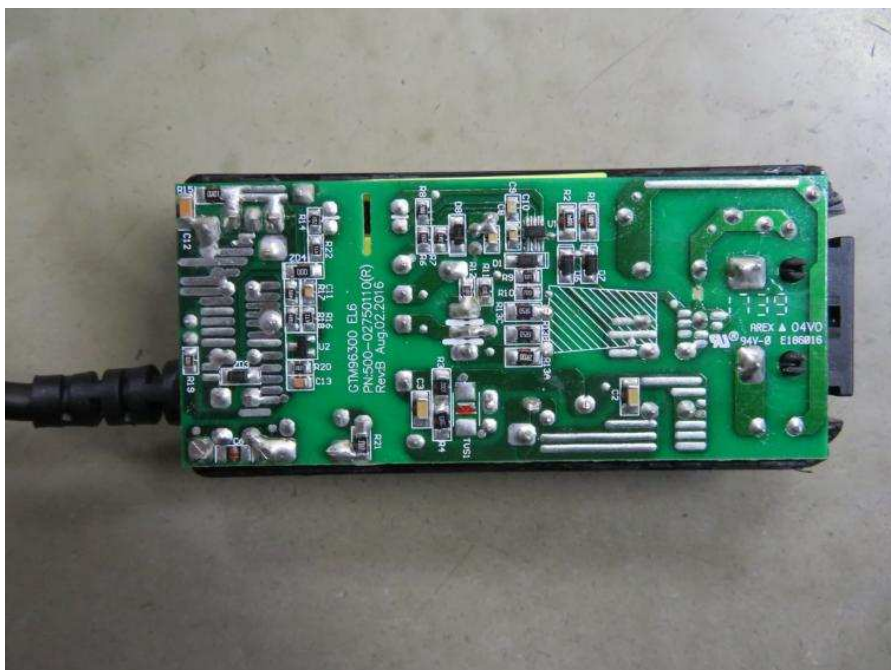
Photo 58 - PCB for GTM96300 series (class II with functional earth)
