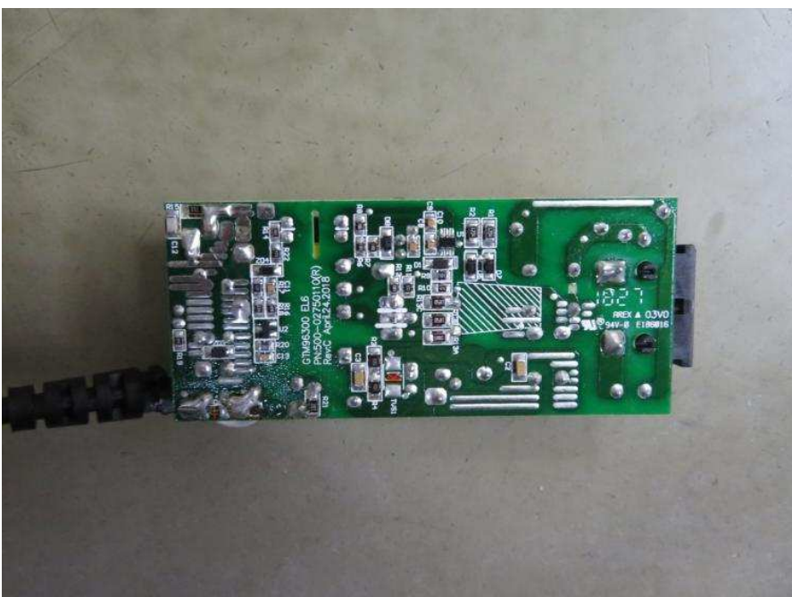
Photo 60 - PCB for GTM96300 series (class II with functional earth)
