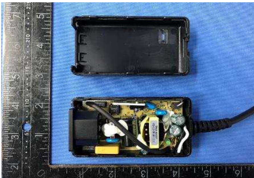
Photo 38 - Internal view for GTM96180 series (Class I) without heatsink for D2
