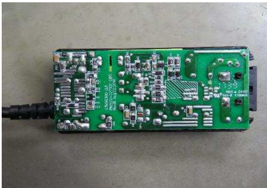
Photo 30 - PCB view for GTM96300 series (class II with functional earth)
