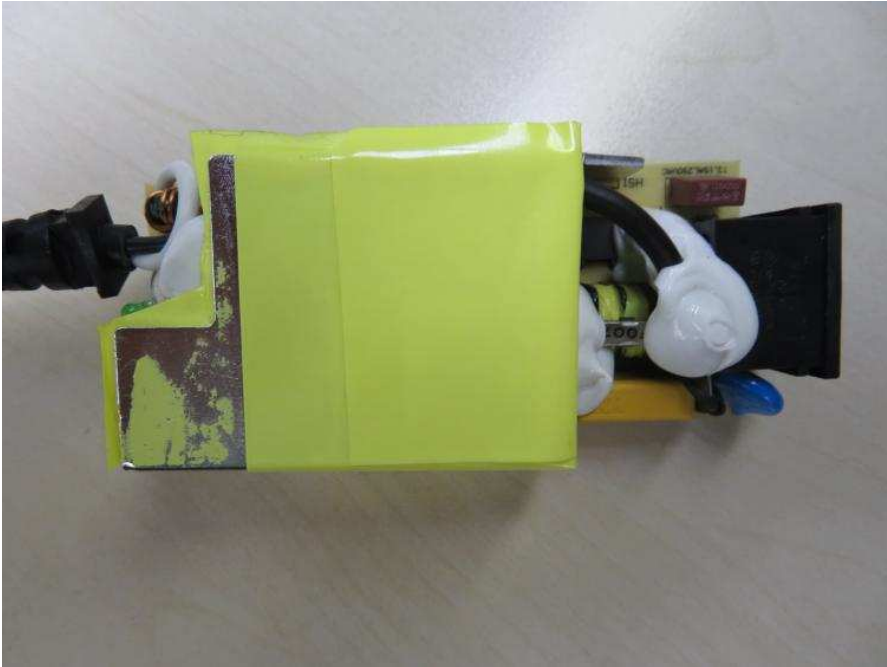
Photo 60 - PCB for GTM96300 series (class II with functional earth)
