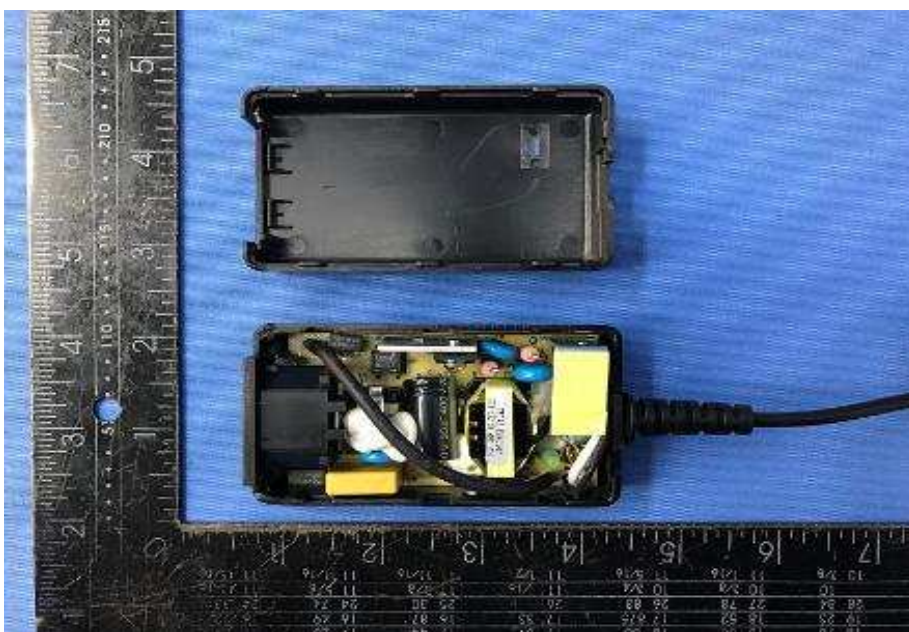
Photo 32 - Internal view for GTM96180 series (Class I) with R22, R23 and without R24
