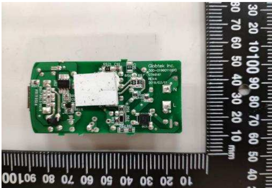
Photo 18 - Bottom view of power board for one USB port
