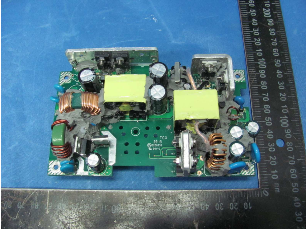
Photo 4: After IP test, internal inspection was performed with gum removed.
