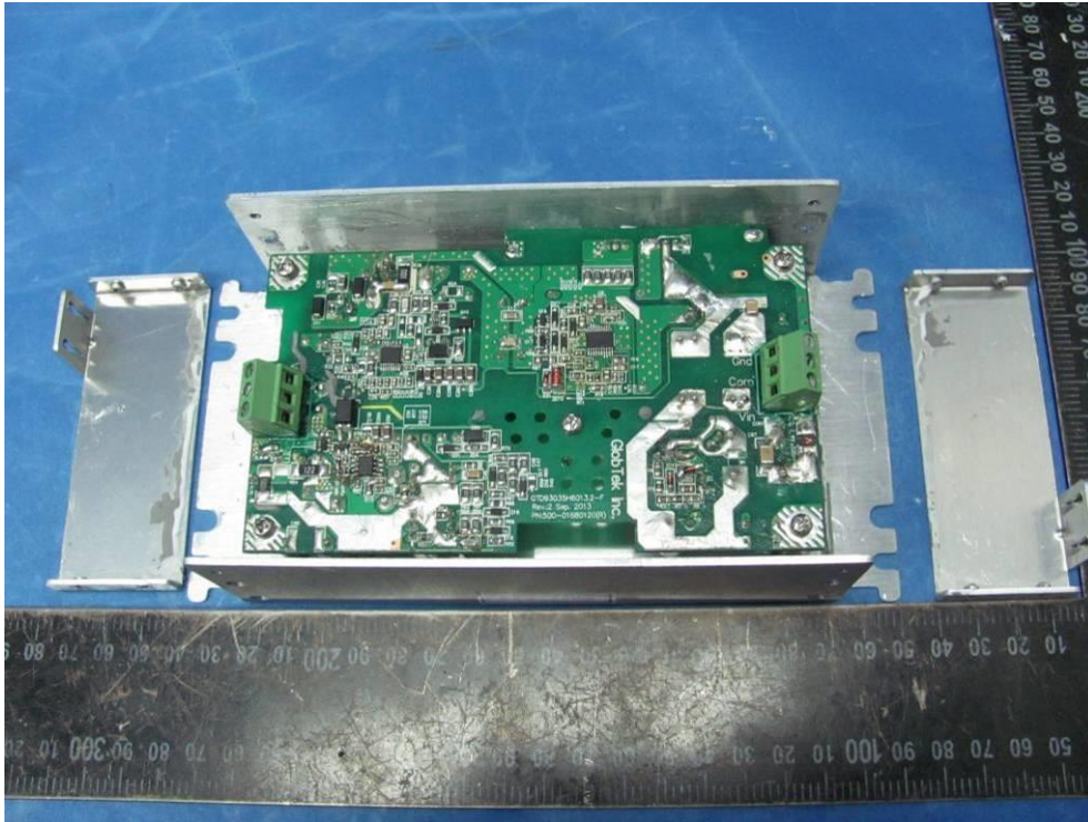
Internal view of EUT_3
