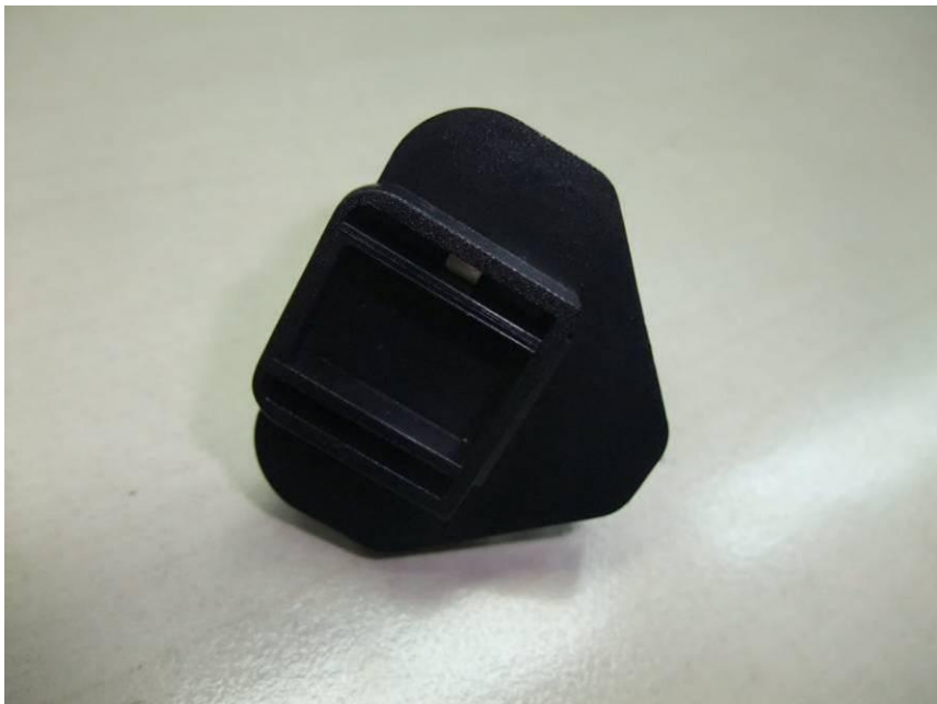
The connector conduct part can't be touched by test finger. CI & CR are measured according to table 2.10.3 & 2.10.4.
