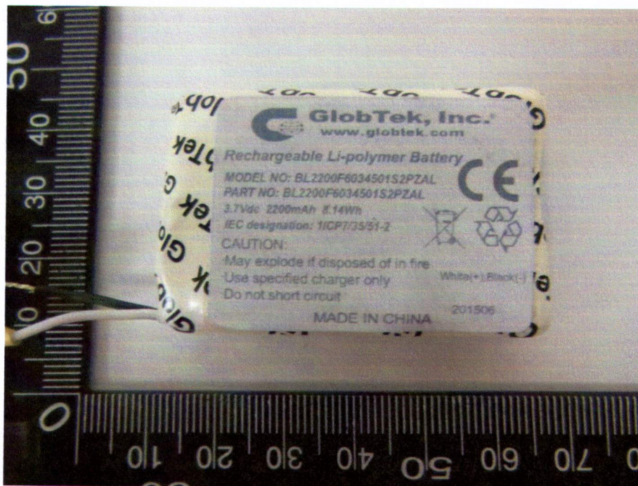
Rechargeable Li-polymer Battery /可充电锂聚合物电池 (3.7Vd.c., 2200mAh, 8.14Wh)
