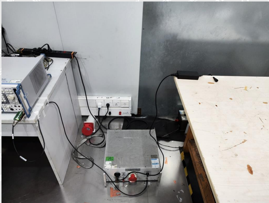
Conduction Emission Test View (TM9-TM10)
