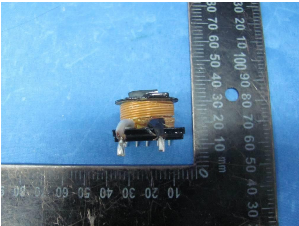
Photo 14: GT*41133 series Secondary winding view of mains transformer (TIW)
