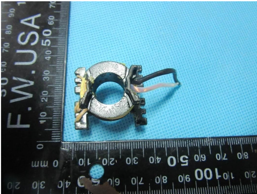
Photo 31: GT*96900P series, GT*961200P series internal view of mains transformer
