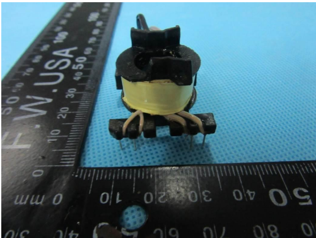
Photo 32: GT*96900P series, GT*961200P series primary winding view of mains transformer
