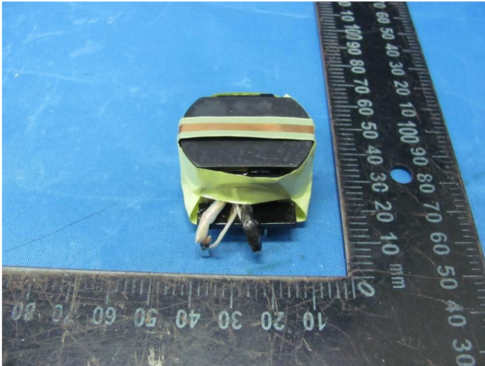
Photo 10: GT*41133 series Pin-out view of mains transformer
