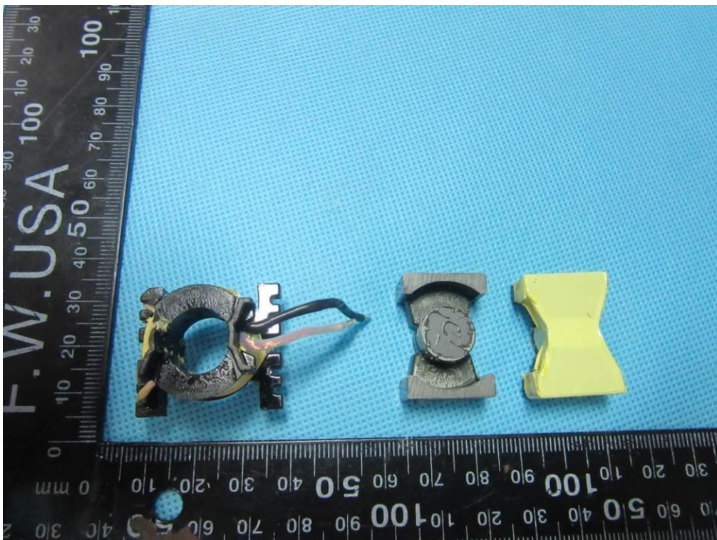
Photo 30: GT*96900P series, GT*961200P series internal view of mains transformer
