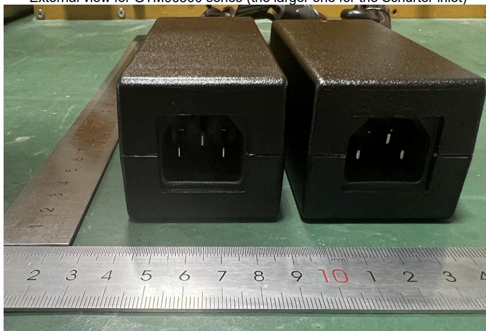
External view for GTM96300 series (the larger one for the Schurter inlet)
