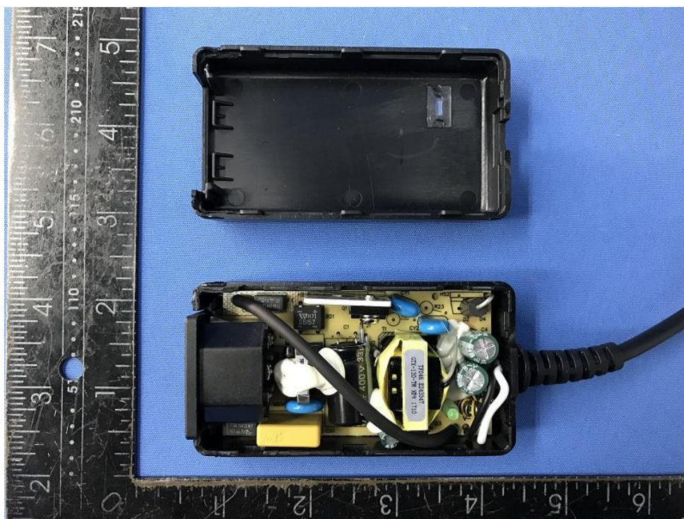
Internal view for GTM96180 series (Class I) without heatsink for D2
