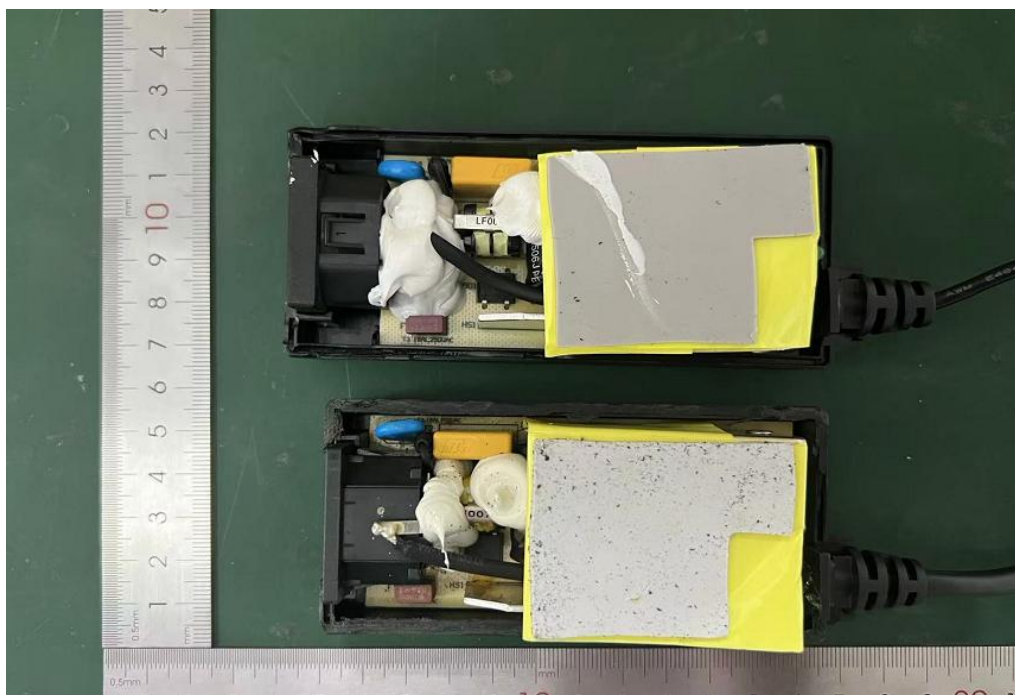
Internal view for GTM96300 series (the larger one for the Schurter inlet)
