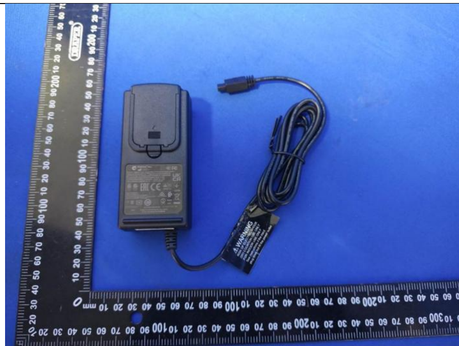
Overall view (plastic enclosure for hybrid desktop) (Secondary voltage > 42V or earthed shall NOT be accessible)
