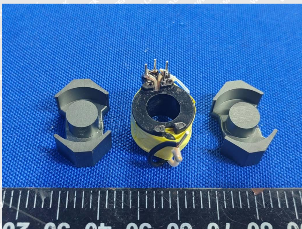
Photo 24 (GTM96183-*PD*-USB1C* Series Transformer – TF123)
