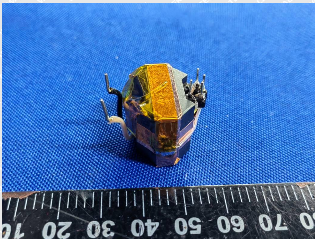
Photo 49 (GTM96181-*PD*** Series Transformer – TF102)
