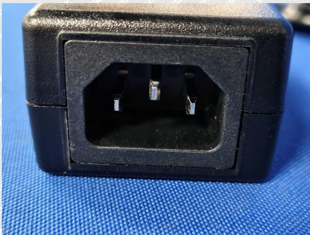
Photo 16 (C14 appliance inlet)
