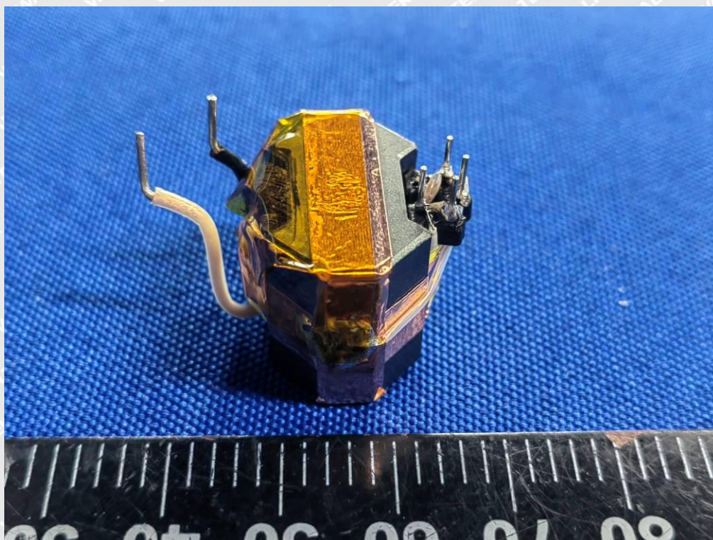
Photo 23 (GTM96183-*PD*-USB1C* Series Transformer – TF123)
