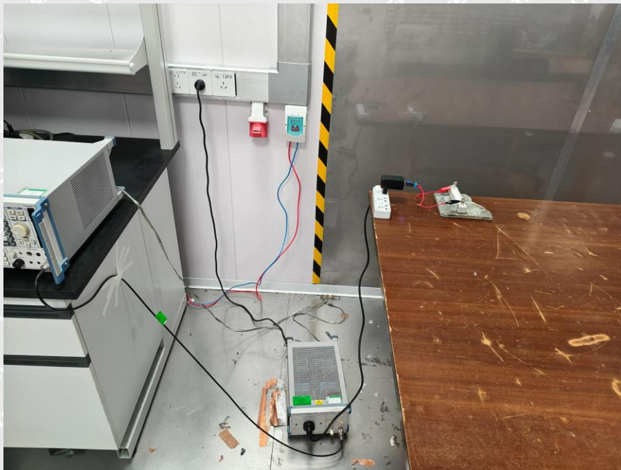
Conducted disturbances from a.c. mains power port
