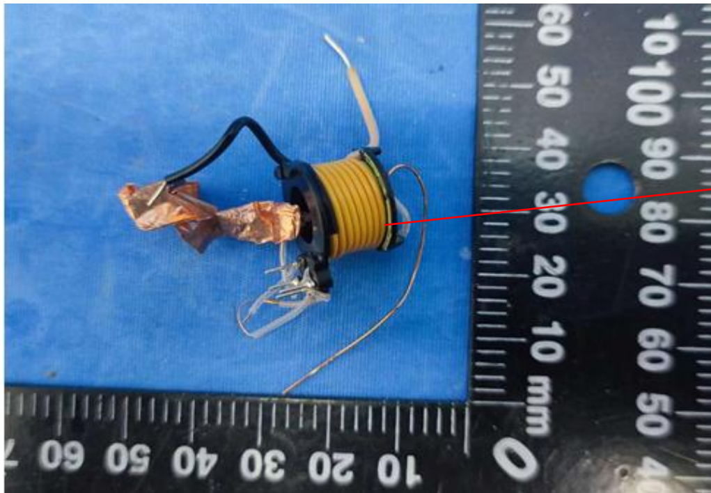
Photo 38 - Transformer view of TF102
