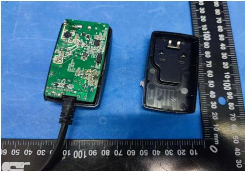
Photo 23 - Internal view of GTM96181-36PD
