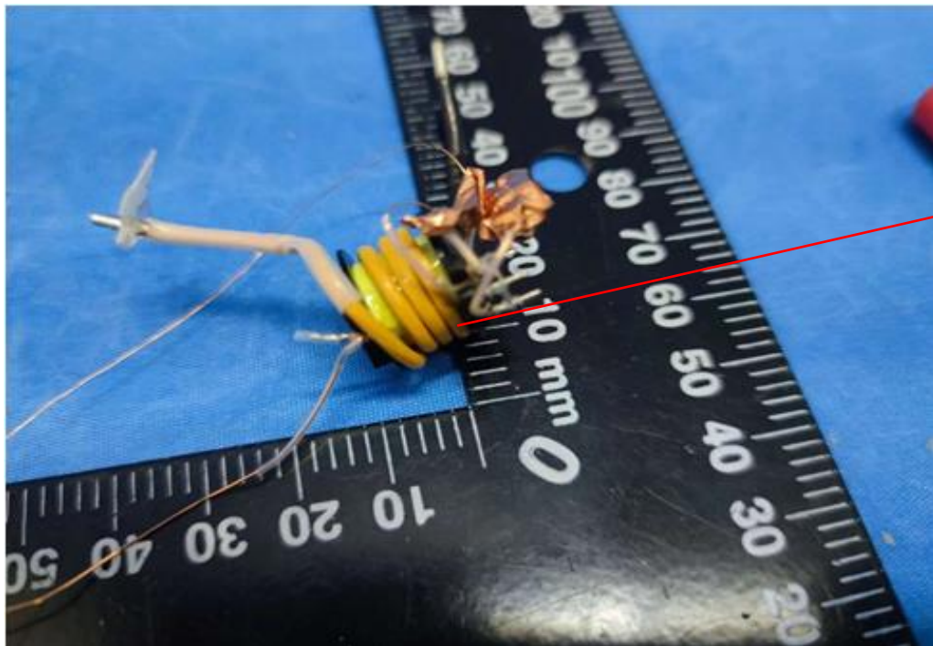
Photo 46 - Transformer view of TF103
