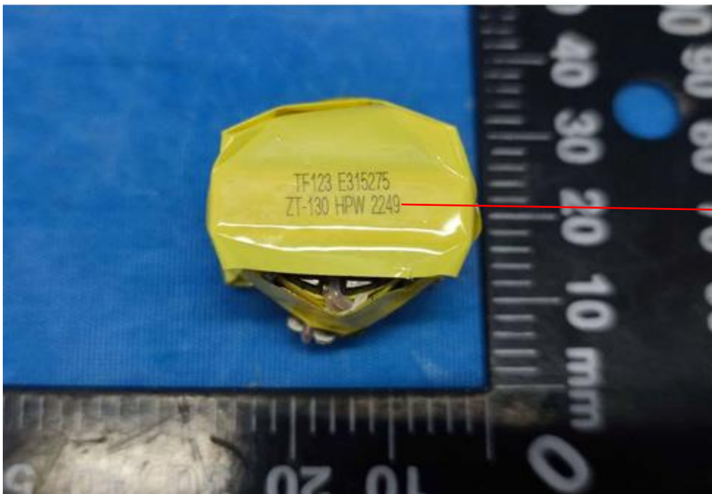
Photo 48 - Transformer view of TF123
