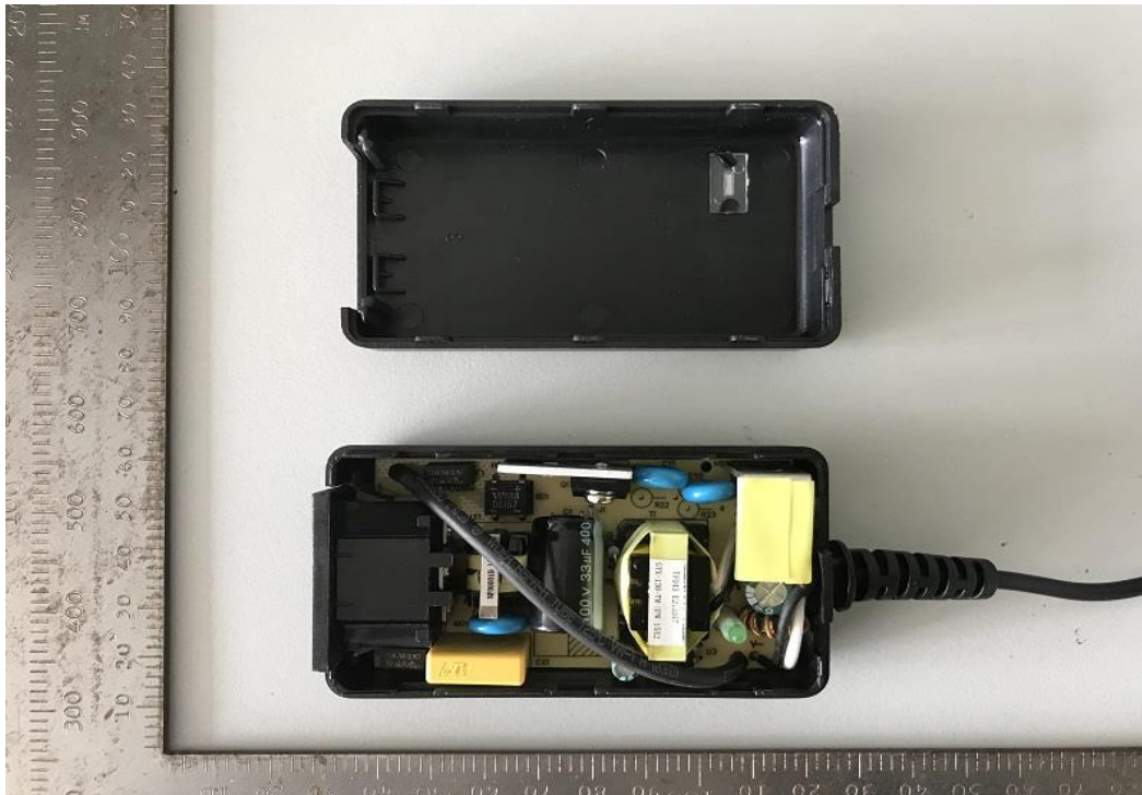
Photo 13 - Internal view for GTM96180 series (Class I) without R22, R23 and R24
