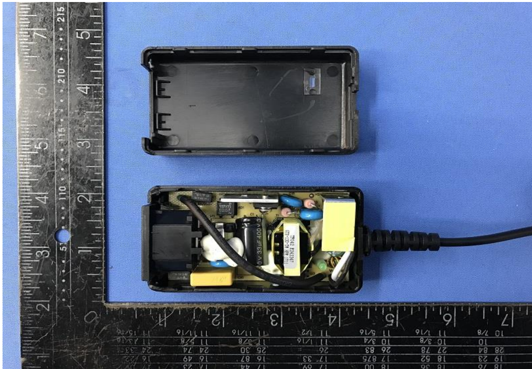
Photo 7 - Internal view for GTM96180 series (Class I) with R22, R23 and without R24
