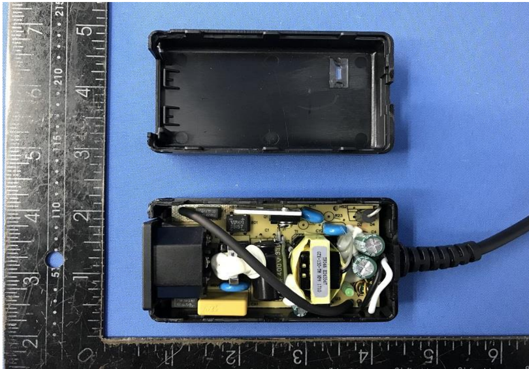
Photo 11 - Internal view for GTM96180 series (Class I) without heatsink for D2
