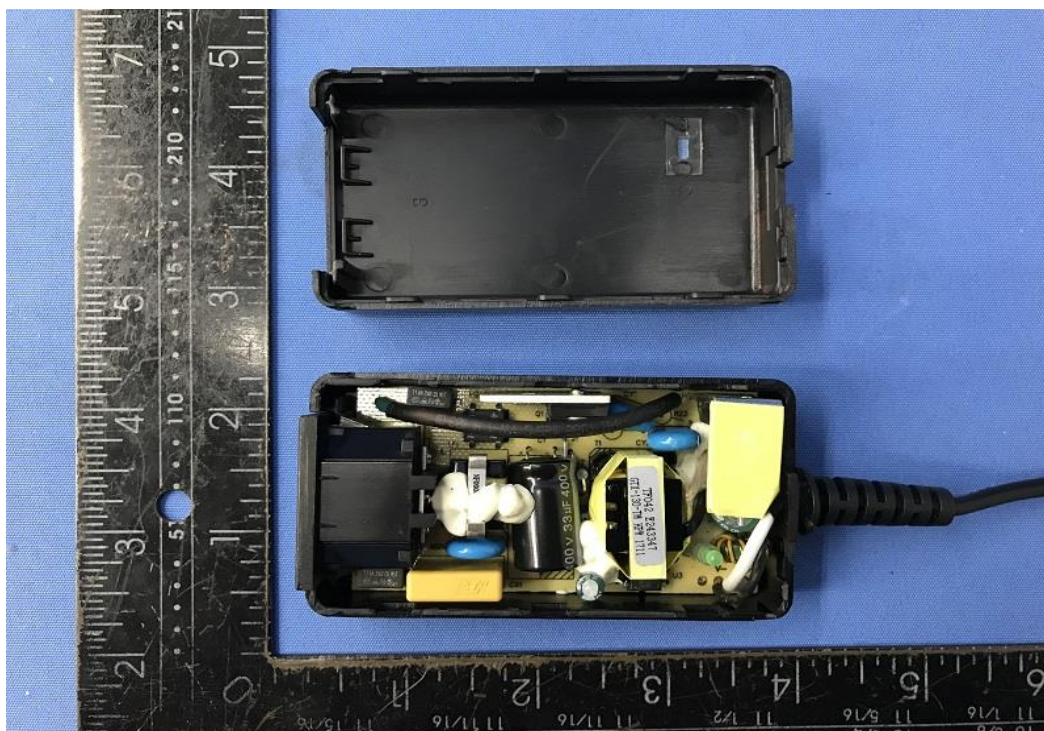
Photo 9 - Internal view for GTM96180 series (Class I) without R22, R23 and with R24
