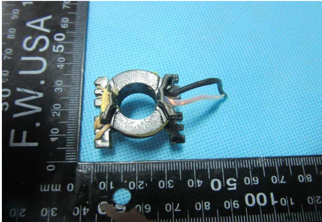
Photo 31 - GT*96900P series, GT*961200P series internal view of mains transformer
