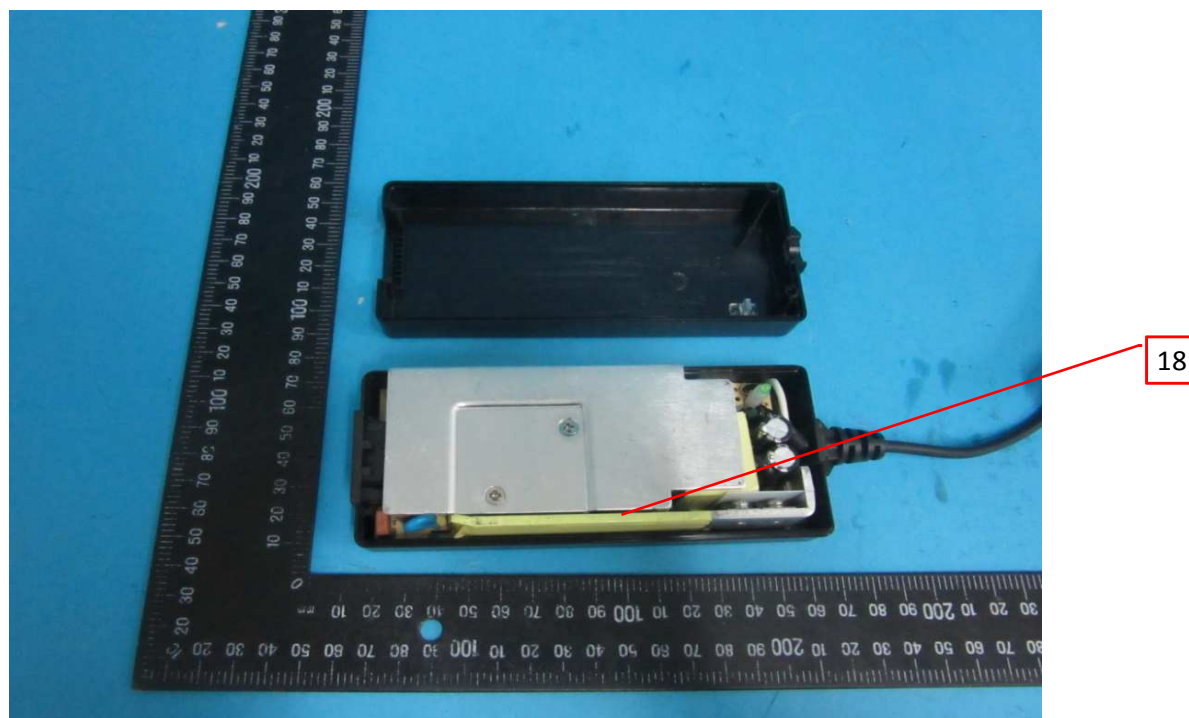
Photo 19 - GT*96900P series, GT*961200P series Internal view of EUT (Class II)
