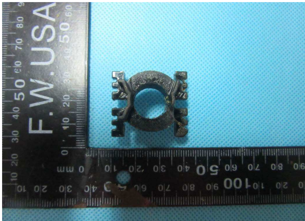
Photo 38 - GT*96900P series, GT*961200P series transformer bobbin
