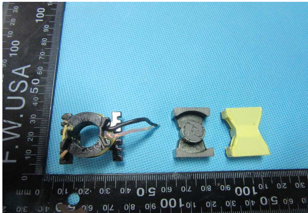
Photo 30 - GT*96900P series, GT*961200P series internal view of mains transformer
