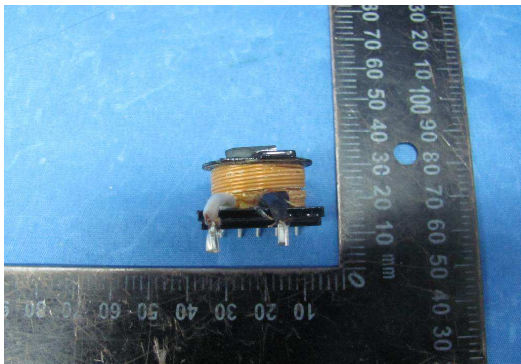
Photo 14 - GT*41133 series Secondary winding view of mains transformer (TIW)
