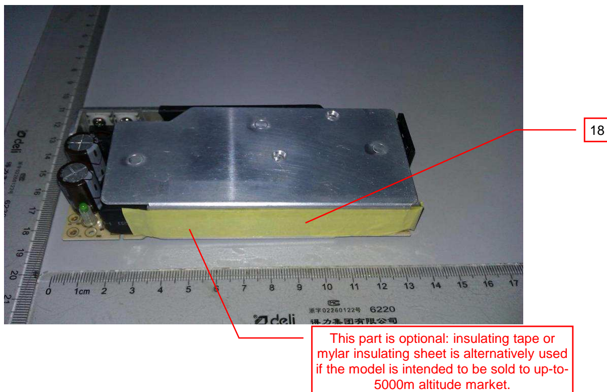
Photo 8 - GT*41133 series View of insulation protection on heatsink (2 layers of insulating tape or 2 layers of heat-shrinkable tube)
