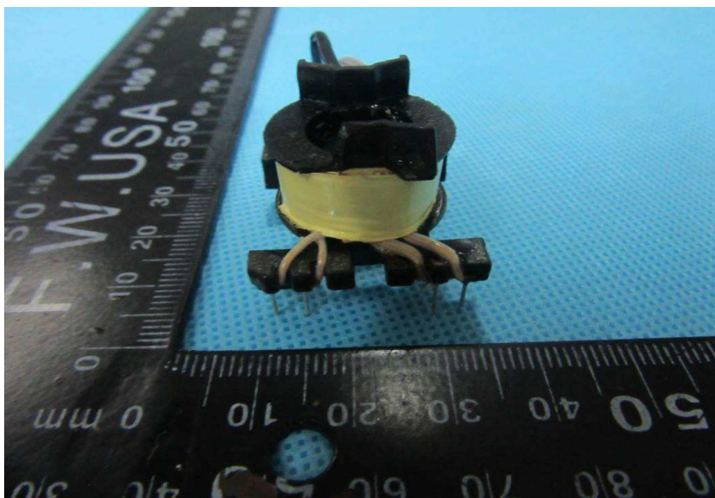
Photo 32 - GT*96900P series, GT*961200P series primary winding view of mains transformer
