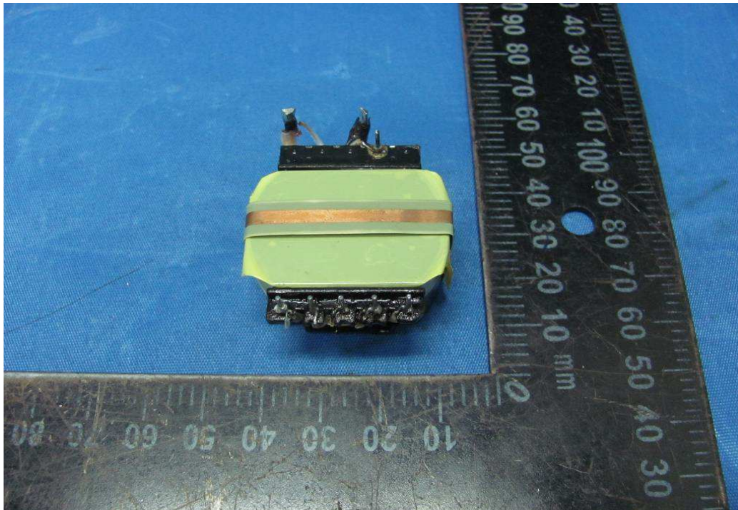
Photo 11 - GT*41133 series External view of mains transformer (shield copper foil)
