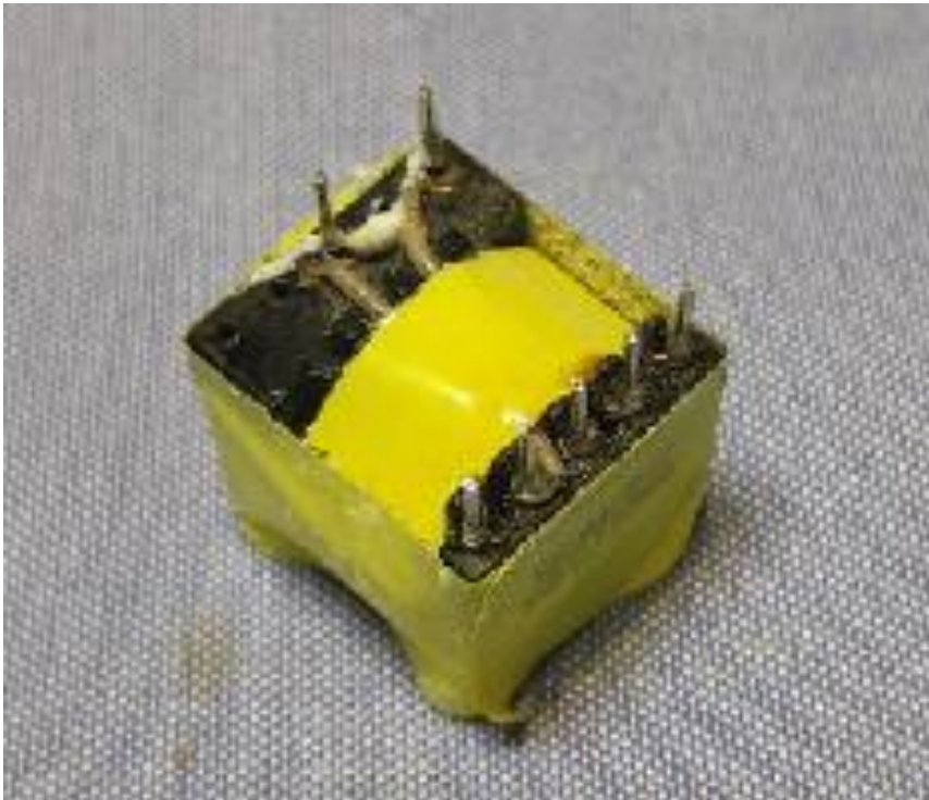
Picture 15 Transformer view
