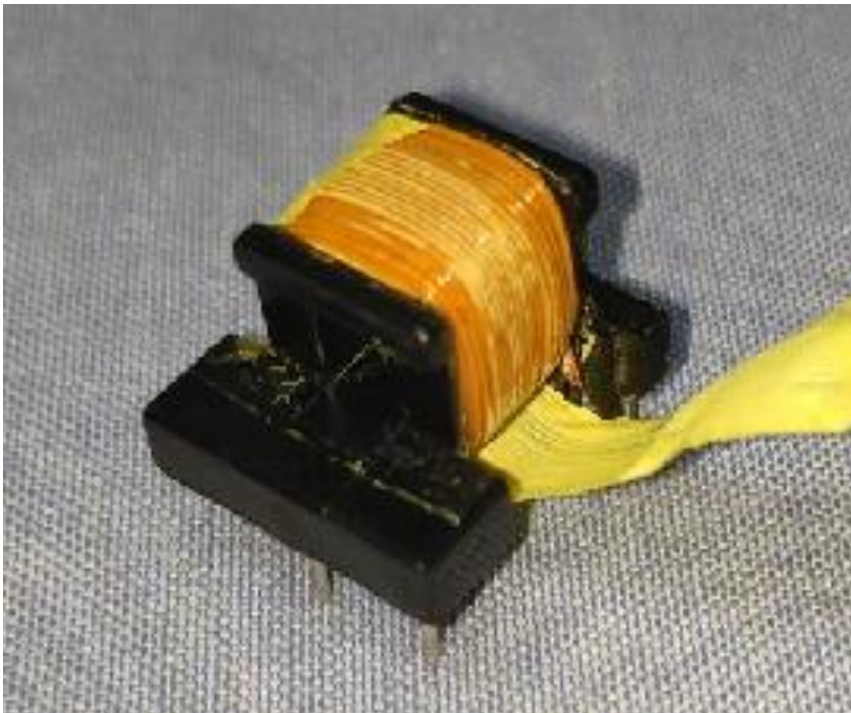
Picture 22 Transformer view
