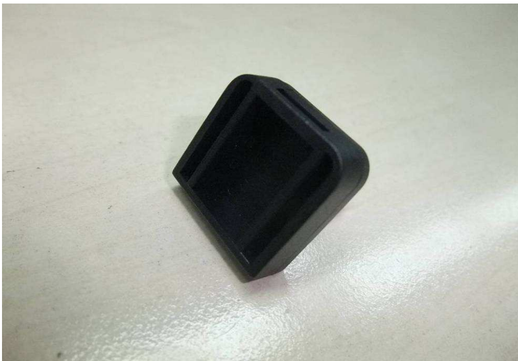
Photo 12 - Connector side view of NEMA 1-15P plug portion
