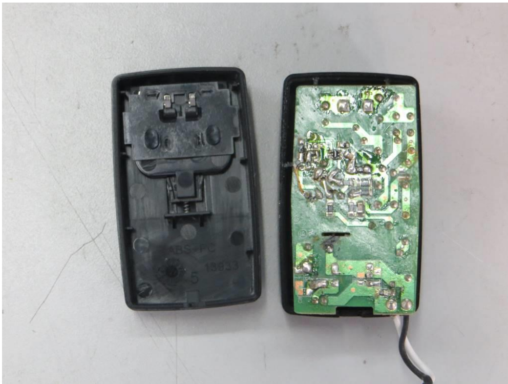
PHOTO 18: Internal view for the structure type only use F1 and a LED indicator (optional)
