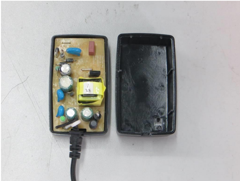
PHOTO 18: Internal view for the structure type only use F1 and a LED indicator (optional)
