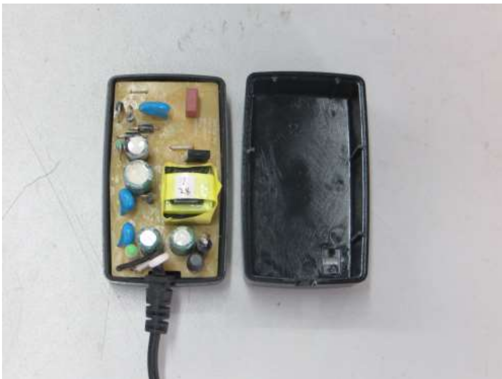
PHOTO 16: INTERNAL VIEW OF ADAPTER MODEL GTM96060 OR GTM41134 SERIES
