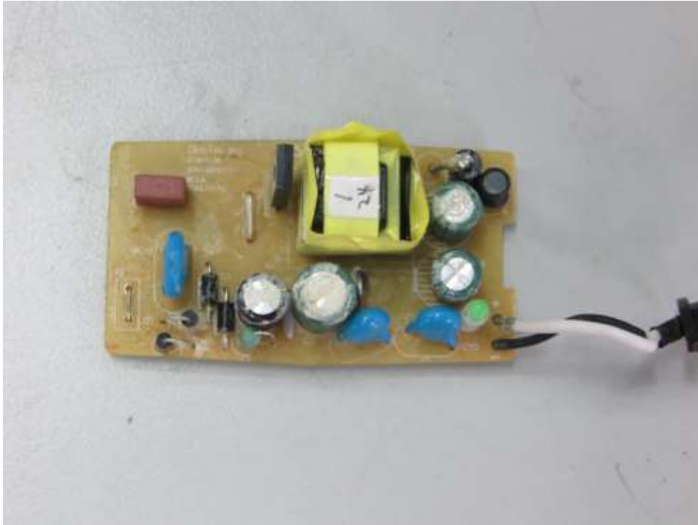
PHOTO 17: COMPONENT SIDE VIEW OF PCB OF MODEL GTM96060 OR GTM41134 SERIES
