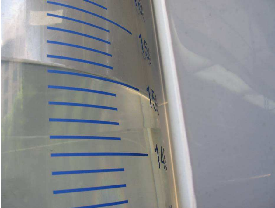
Photo 3: The depth of immersion tank (The lowest point of enclosures is located 1 500 mm below the surface of the water.)
