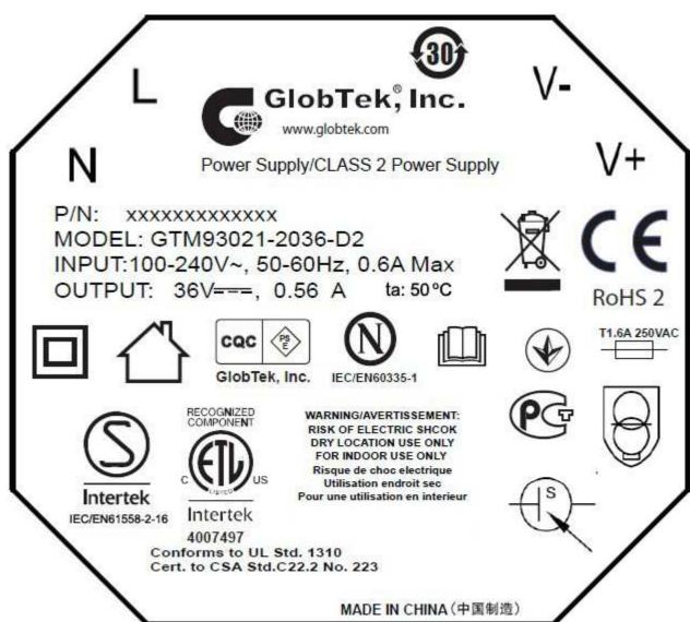
Note: Other models of GT\*93021-\*\*\*-D2 and all models of GT\*93021-\*\*\*-T2 are with similar label as GTM93021-2036-D2 except different model name and output ratings.
