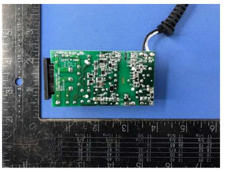
PCB view for GTM96180 series (Class I) with R22, R23 and without R24
