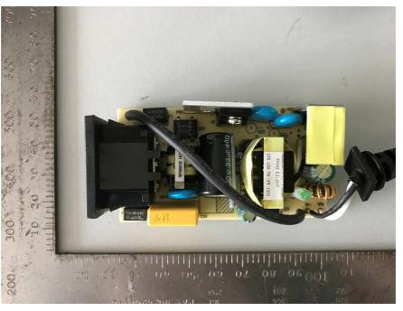
PCB view for GTM96180 series (Class I) without R22, R23 and R24
