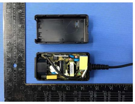
Internal view for GTM96180 series (Class I) with R22, R23 and without R24
