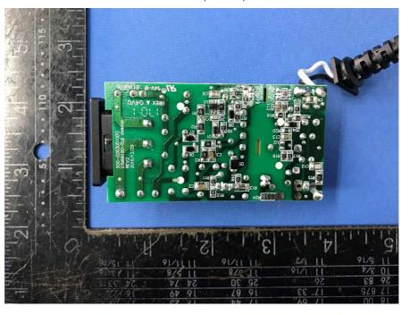
PCB view for GTM96180 series (Class I) without heatsink for D2
