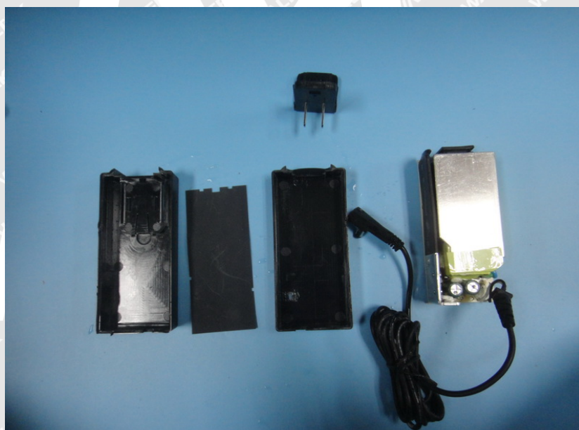
Photo 2 -- After the test for IPX2
