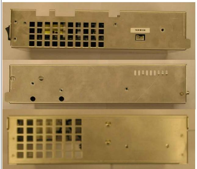
Marking plate is provided on the back side of the enclosure. It is not visible when the power supply unit is build-in the end medical product. Type and fuse rating of external accessible fuses is provided on the front side of the enclosure.
