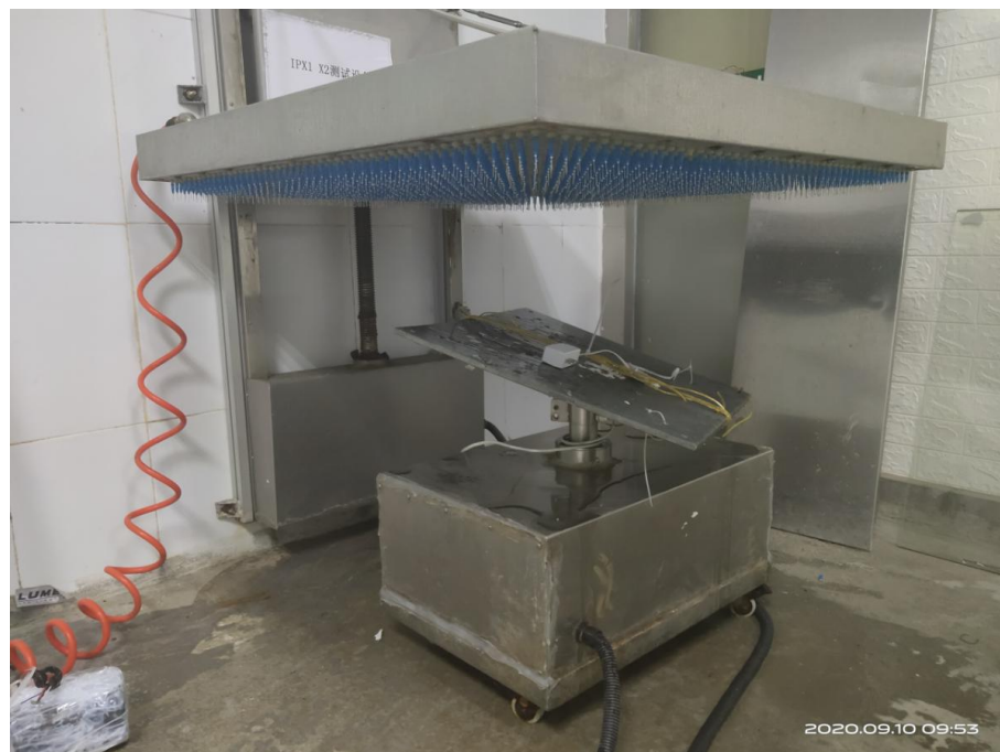
Photo 8: IPX2 test of model GT*86100-**-W2*
