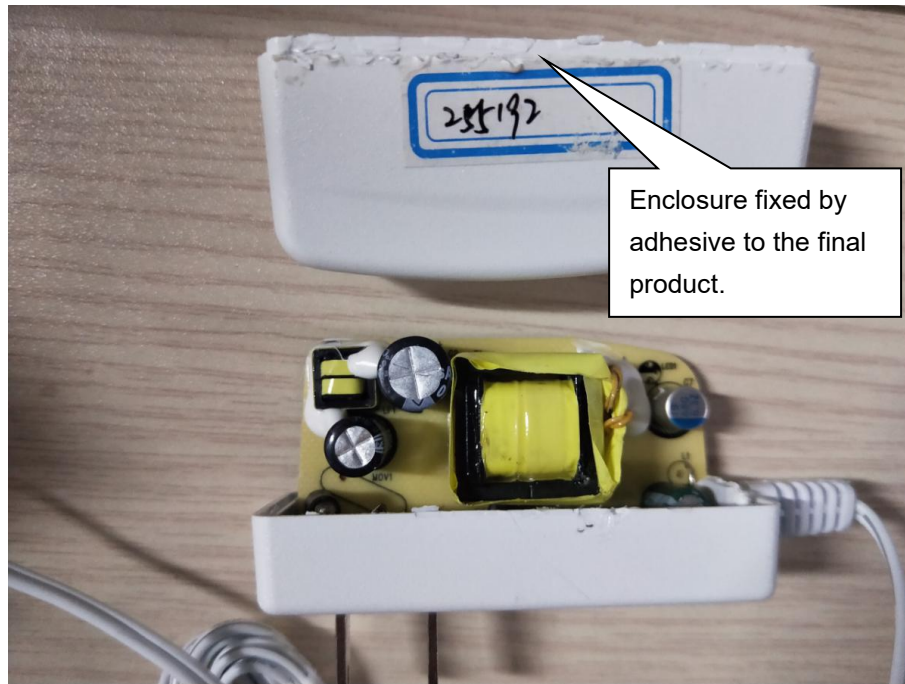
Photo 11: Test result after IP2X and IPX2 test
