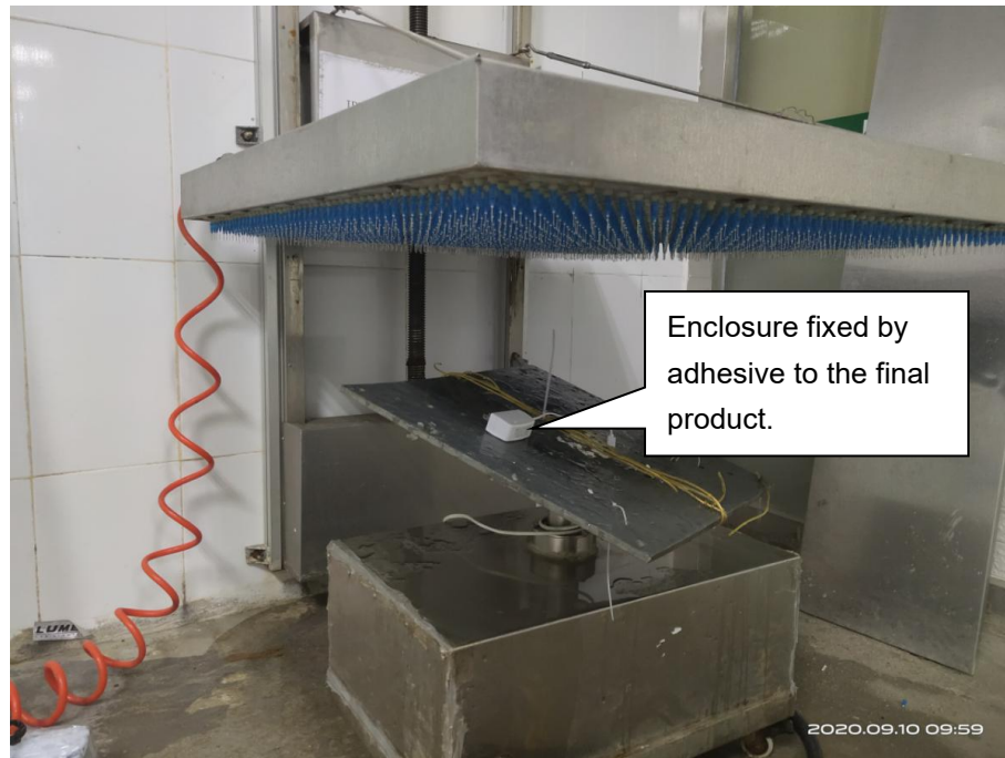
Photo 7: IPX2 test of model GT*86100-**-W2*
