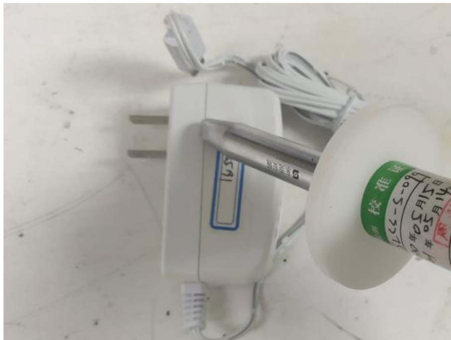
Photo 6: IP2X test of model GT*86100-**-W2*
