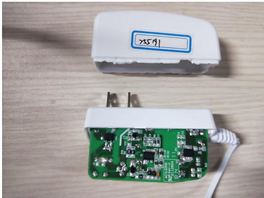
Photo 10: Test result after IP2X and IPX2 test
