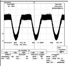
Input voltage: 240Vac; 60Hz Test Condition was: rated load
