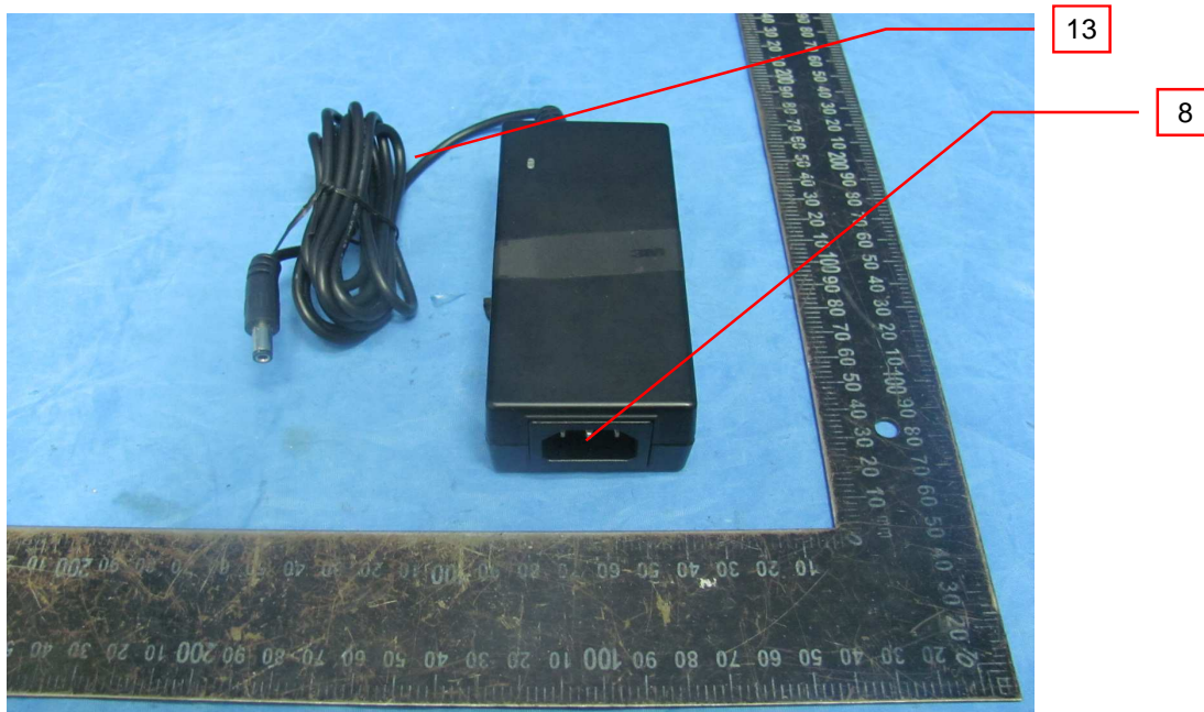
Photo 7 - External view for GTM96600 series (Class I)
