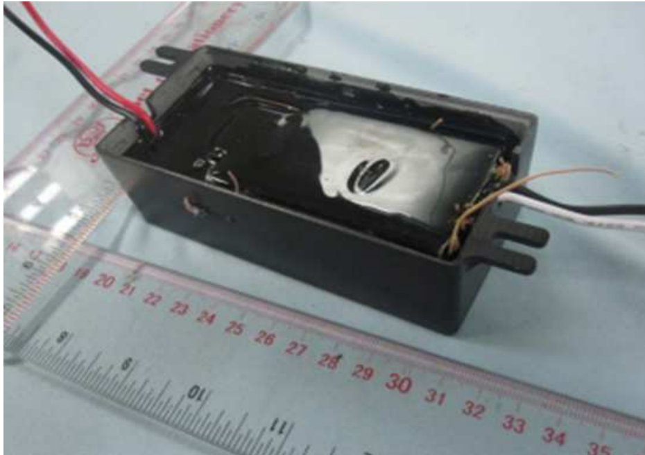
Photo 12 - Internal view for GTM91099 series (Encapsulated)
