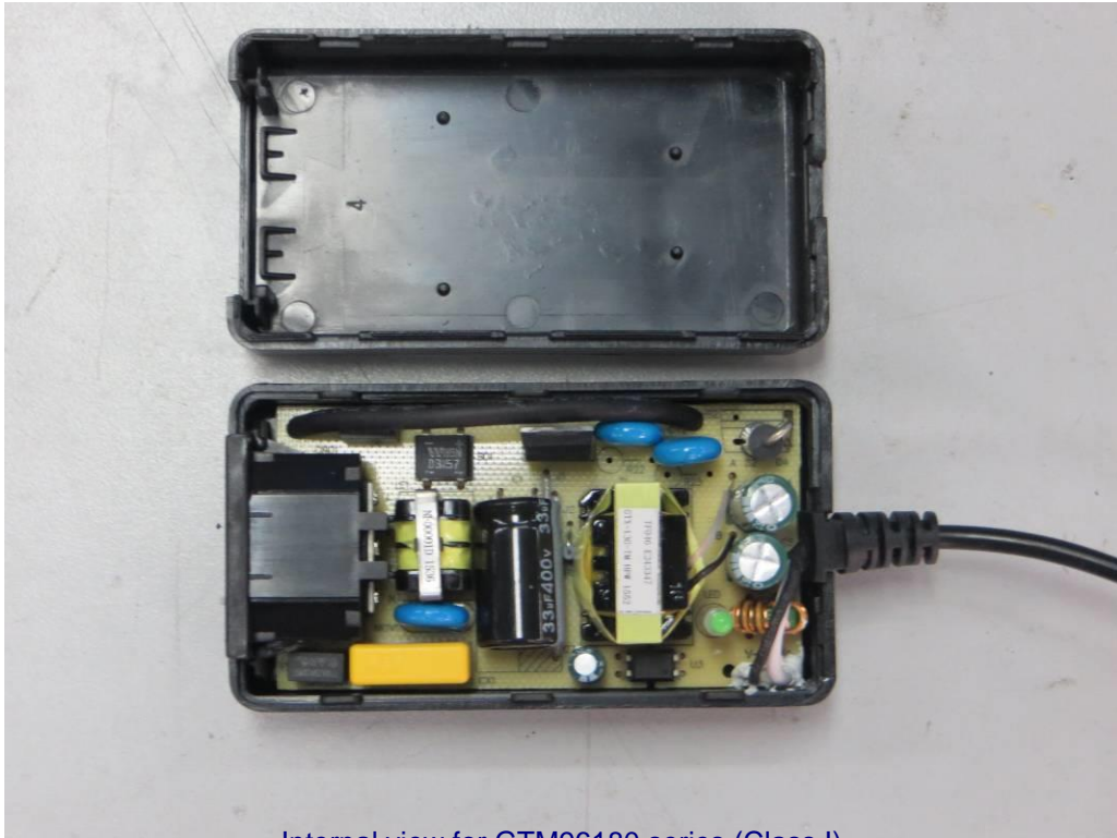
Internal view for GTM96180 series (Class I)
