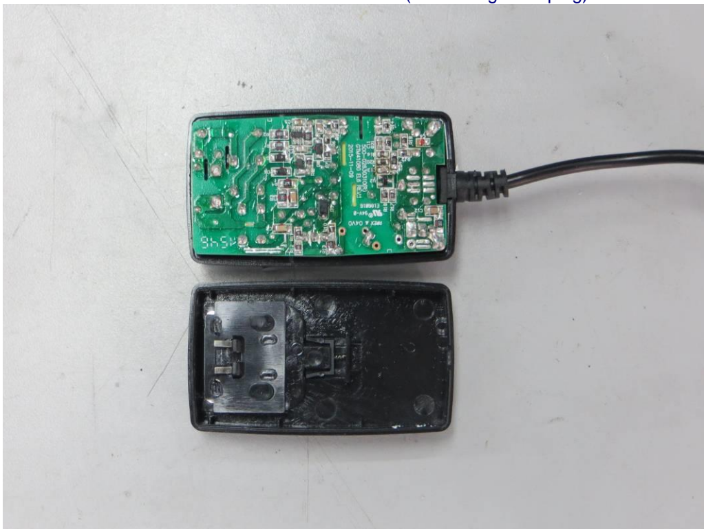
Internal view for GTM96180 series (Interchangeable plug)
