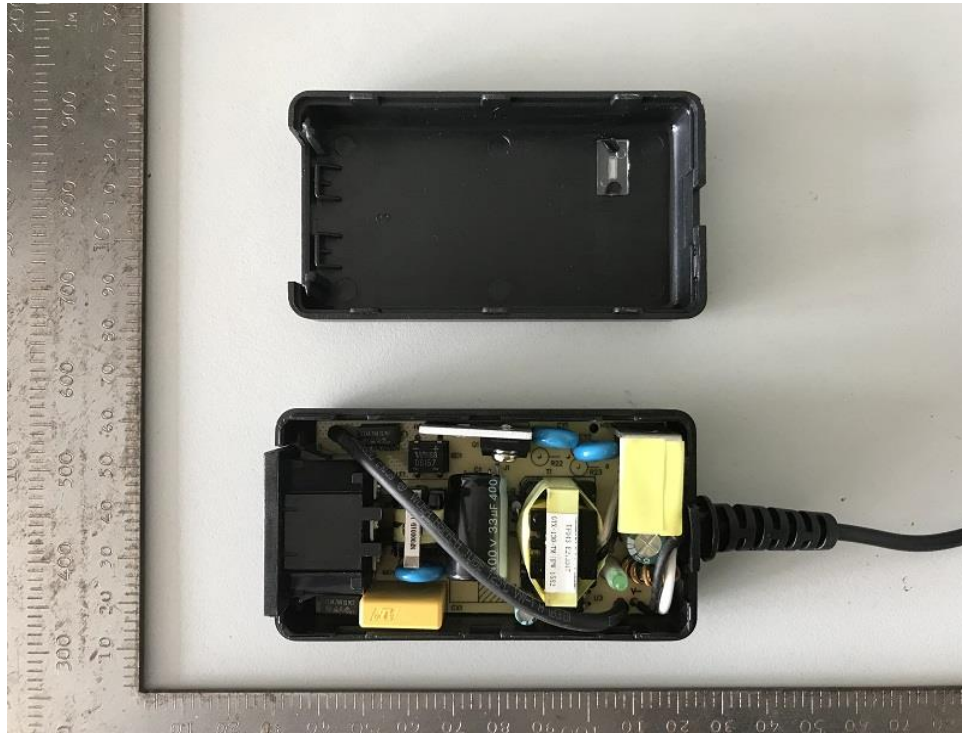
PCB view for GTM96180 series (Class I) without R22, R23 and with R24
