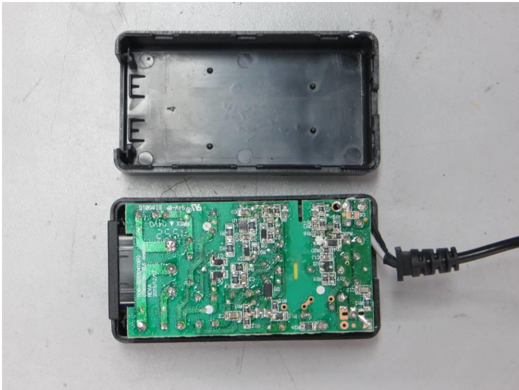
Internal view for GTM96180 series (Class I)
