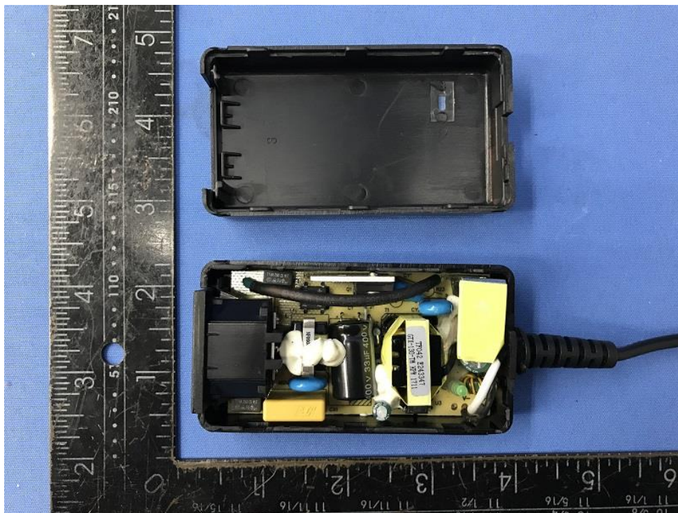
Internal view for GTM96180 series (Class I) without R22, R23 and with R24
