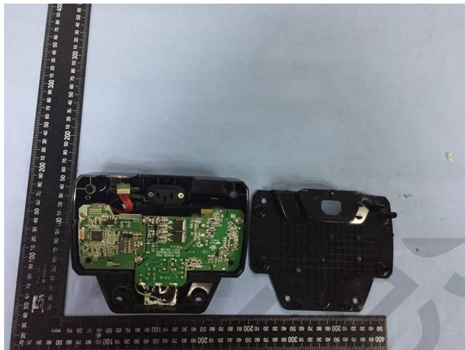
**Solder Board-Component View 1**
