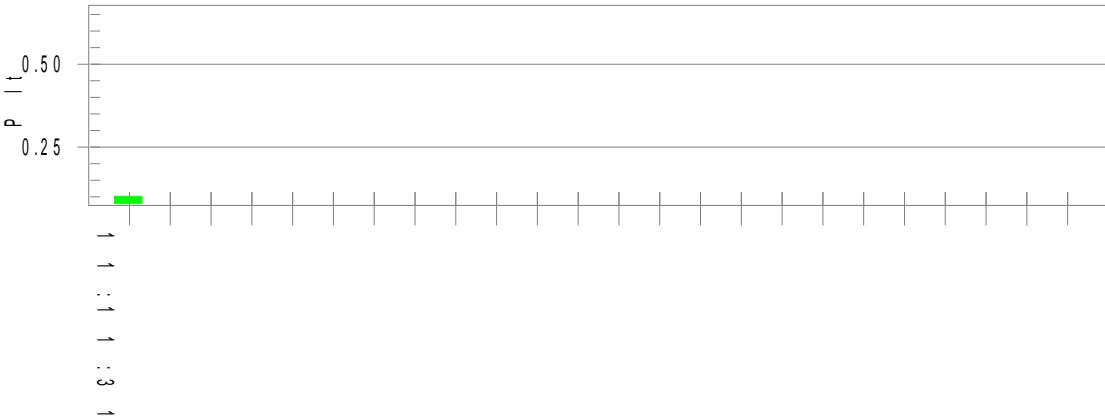
**Parameter values recorded during the test:****Vrms at the end of test (Volt):** 229.84**Highest dt (%):****T-max (mS):** 0**Test limit (%):****Test limit (mS):** 500.0 **Pass****Highest dc (%):** 0.00**Test limit (%):** 3.30 **Pass****Highest dmax (%):** 0.00**Test limit (%):** 4.00 **Pass****Highest Pst (10 min. period):** 0.233**Test limit:** 1.000 **Pass****Highest Plt (2 hr. period):** 0.102**Test limit:** 0.650 **Pass**
