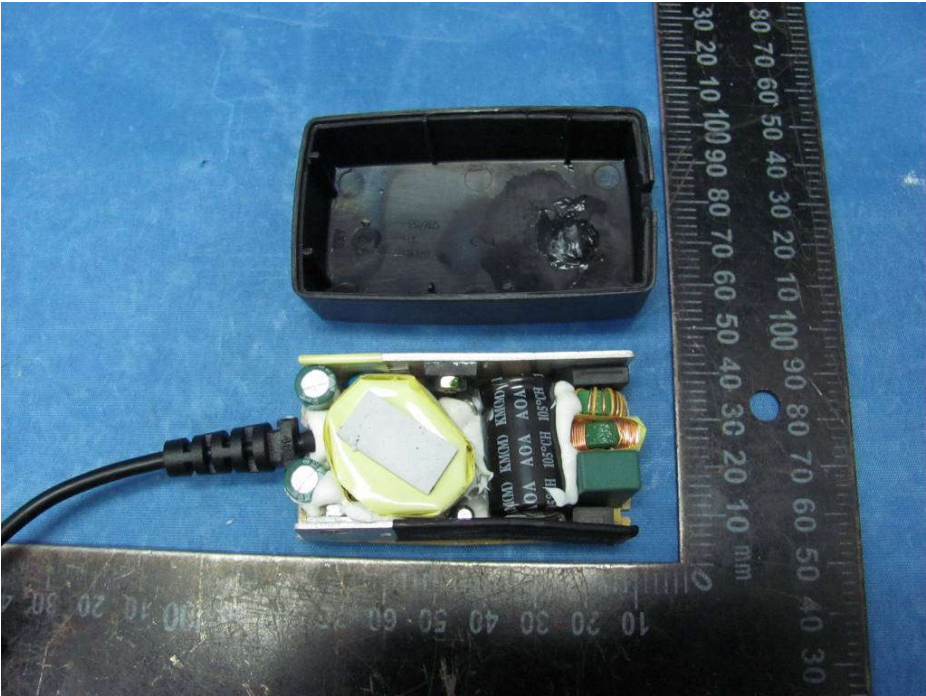
Fig. 4 - Internal view – Component side view of PCB
