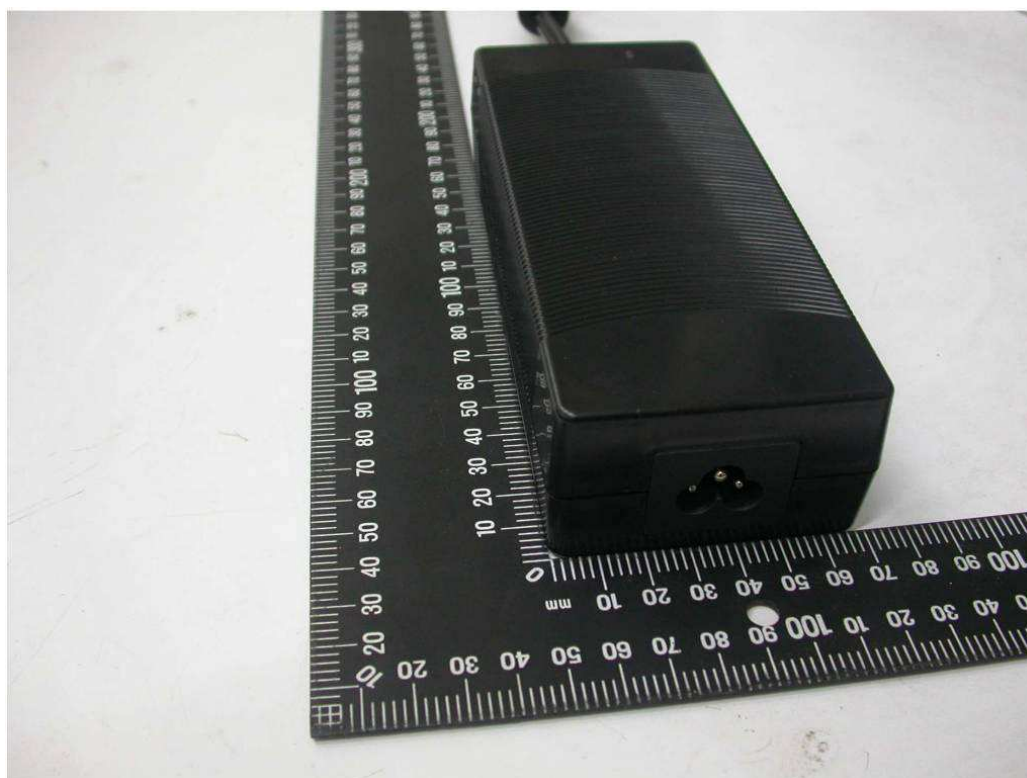
Fig. 2 - External view - 2 of EUT with appliance inlet complied with standard sheet C6 of IEC 60320
