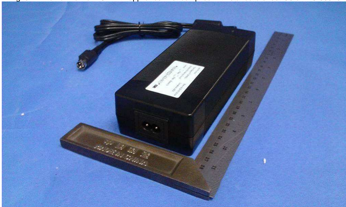
Fig. 3 – External view of EUT with appliance inlet complied with standard sheet C8 of IEC 60320
