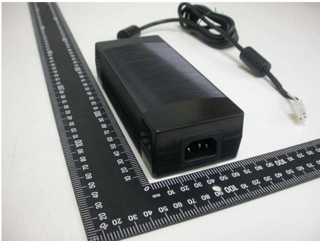
Fig. 2 - External view - 2 of EUT with appliance inlet complied with standard sheet C6 of IEC 60320
