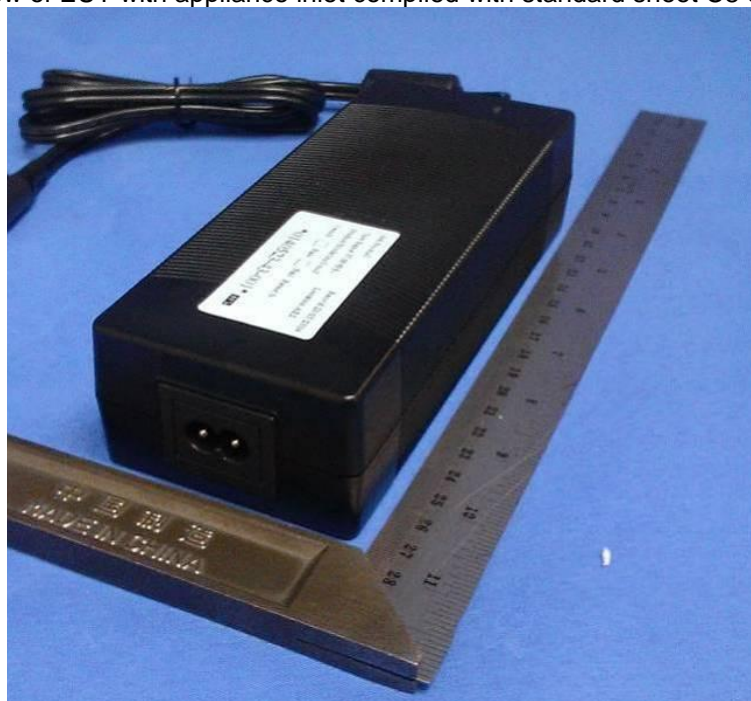
External view of EUT with appliance inlet complied with standard sheet C8 of IEC 60320
