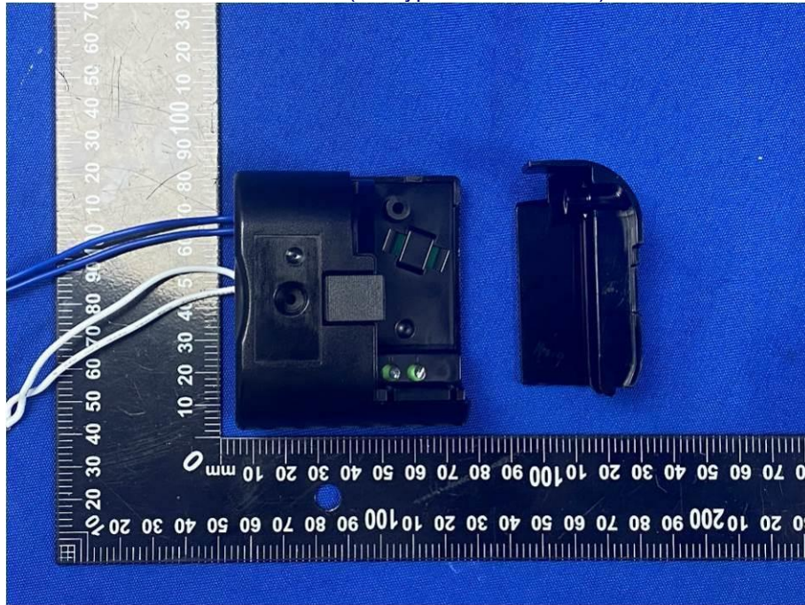
Internal view (for Type A construction)
