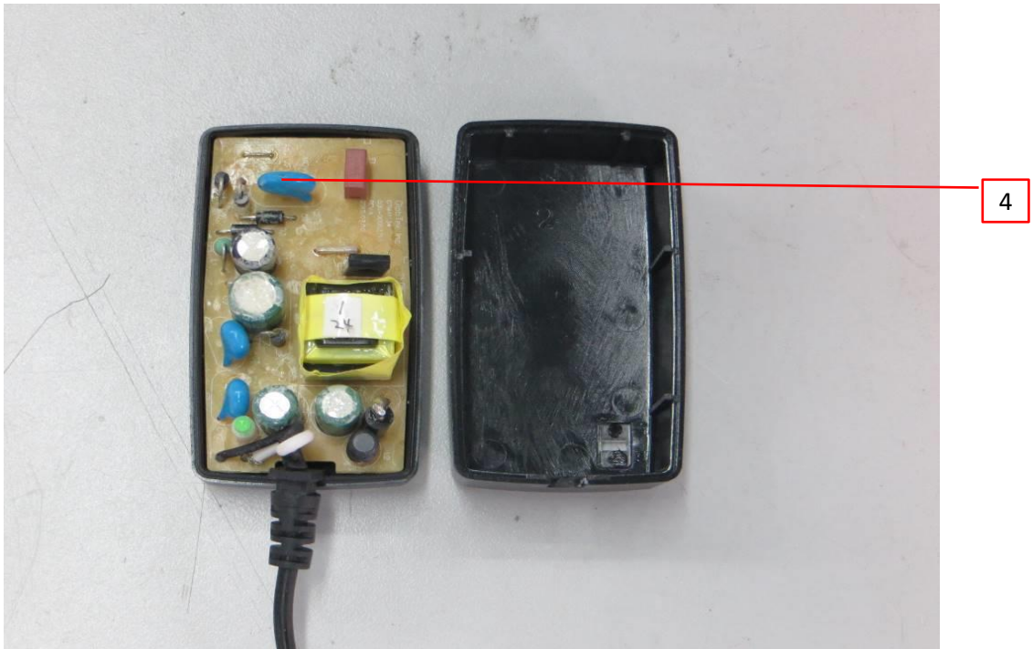
Photo 9 - Internal view for the structure type only use F1 and a LED indicator (optional)
