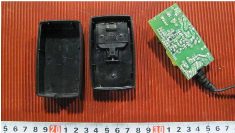
PHOTO 4: INTERNAL VIEW OF ADAPTER MODEL GT*41134-***
