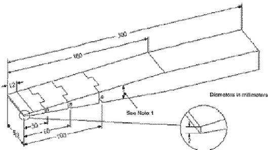
Figure JA.2 Wedge-probe
