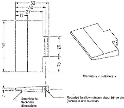
Figure JA.2 Wedge-probe
