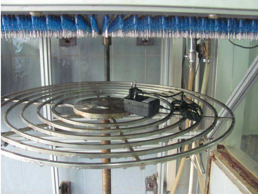
Photo 7: IPX1 test for EUT
