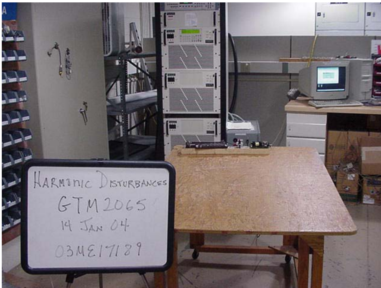
Harmonic Disturbances and Flicker Test Set-Up
