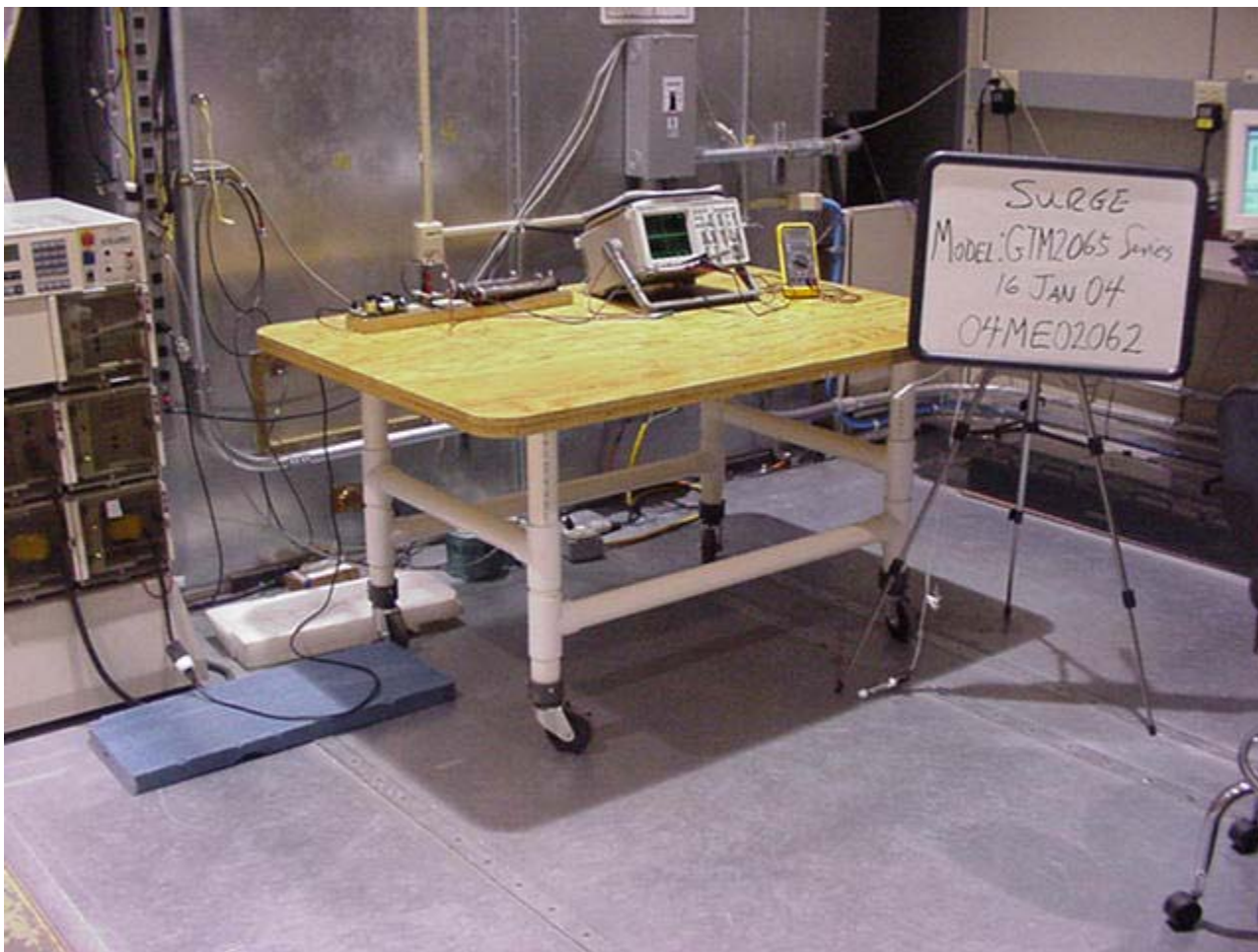
Voltage Surge Test Set-Up
