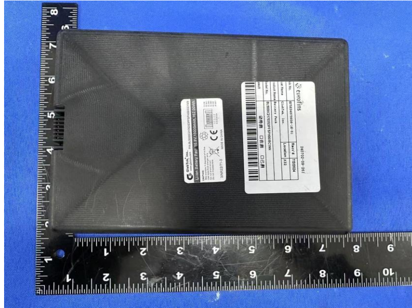
Photo 47 Overview of battery for 3S3P- Battery with case
