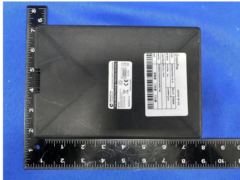
Photo 43 Overview of battery for 2S3P- Battery with case
