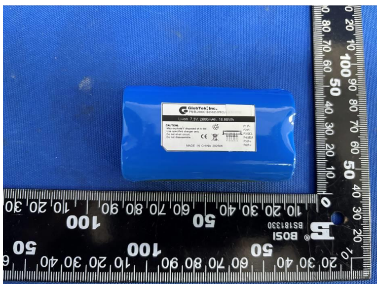
Overview of battery (BL2600C186502S1PFCU)
