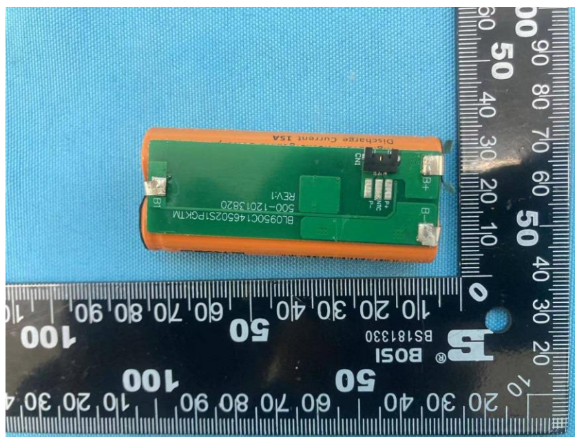
Battery internal view for BL0950C146502S1PGKTM
