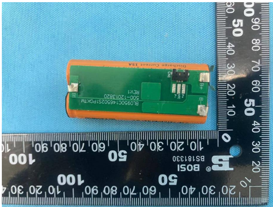
Battery internal view for BL0950C146502S1PGKTM
