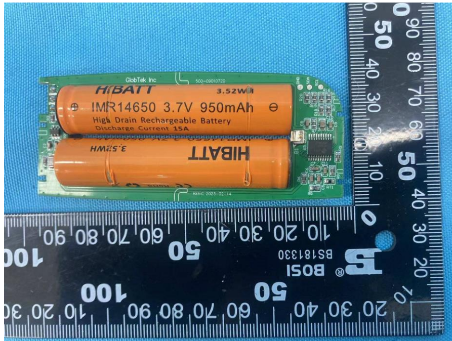
Battery internal view for BL0950CAA652S1PFCT
