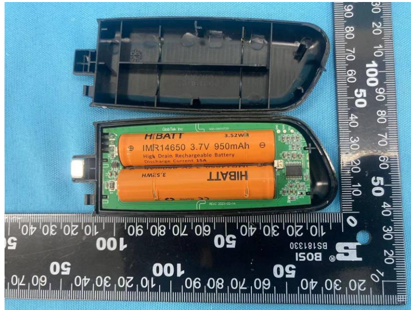
Battery internal view for BL0950CAA652S1PFCT
