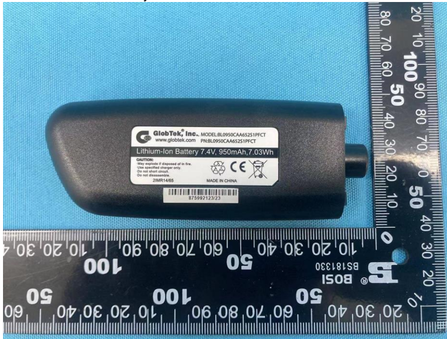
Photo 1. Battery view for BL0950CAA652S1PFCT
